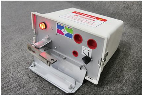
The indicator will flash when safety circuit was broken
